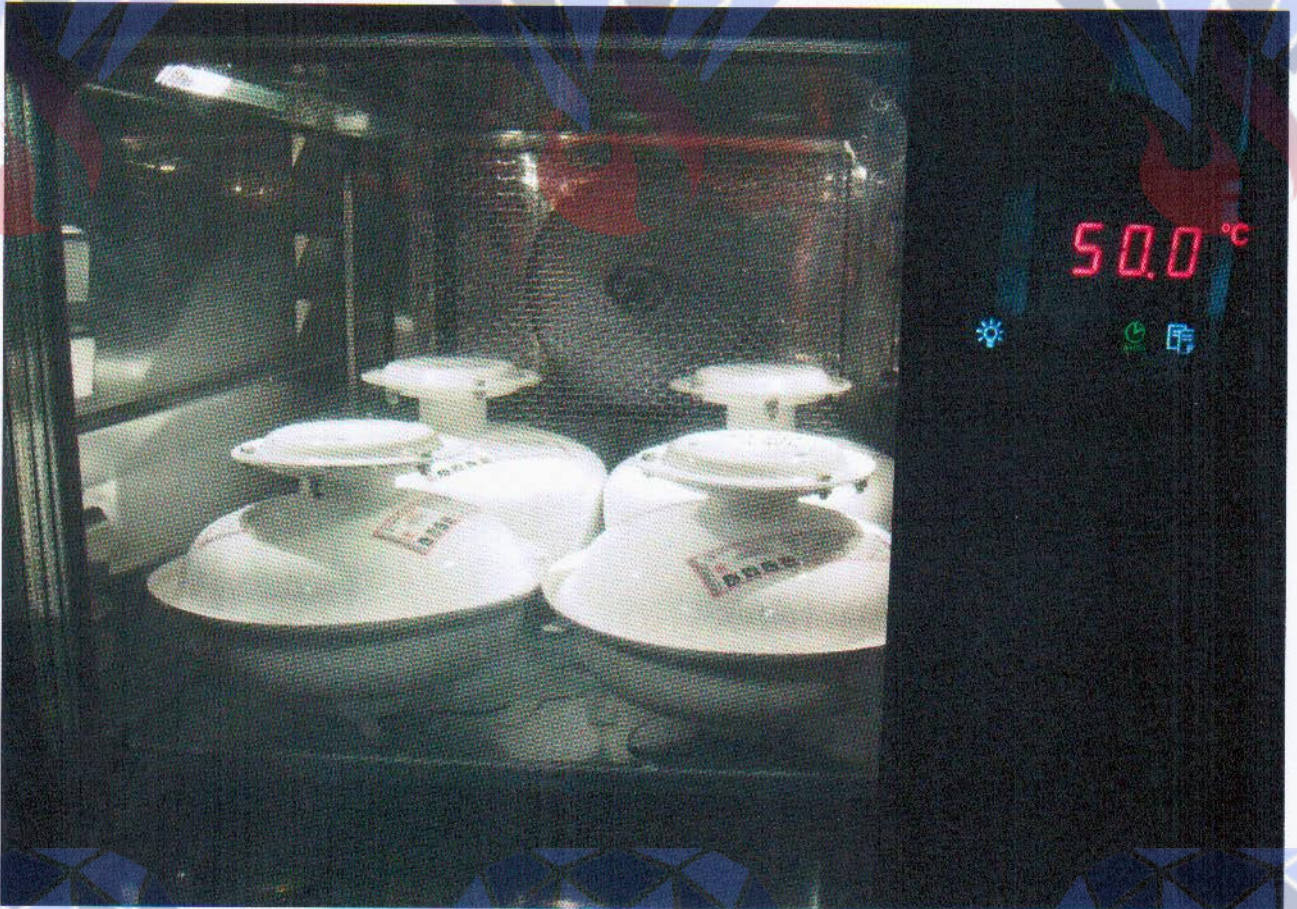
Fig. No. 9 and 10: The module samples in the climatic chamber during the test acc. to 4.6.
